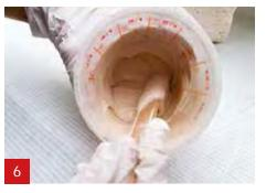
Thix A has been added to the A1 to get a thick texture, which can be formed and sanded.
