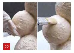
The C-veil must be covered with a layer of A1 by hand or brush.
