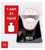
Weigh 1 part of A1 liquid. In this example we use 100 g A1 liquid.
