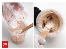
Add as much ATP powder as needed into the A1. Stir firmly till all lumps have disappeared.
