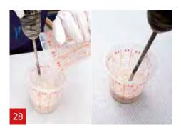
Gently add the A1 powder to the A1 liquid. Stir the mixer till all lumps have disappeared (± 1 min.) resulting in a smooth material.
