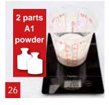
Weigh 2 parts of A1 powder. In this example we used 200 g A1 powder.
