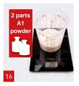
Weigh 2 parts of A1 powder. In this example we use 200 g A1 powder.
