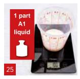
Weigh 1 part of A1 liquid. In this example we used 100 g A1 liquid.
