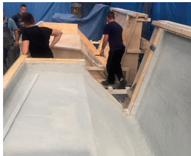
A1 element laminated in the mould
