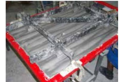
A frame is used to position the mounting brackets on the finished laminate.
