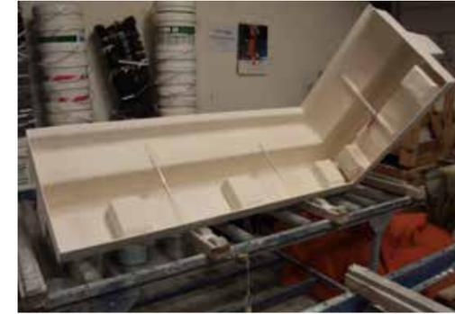
On the inside panels are being reinforced with aluminum.
