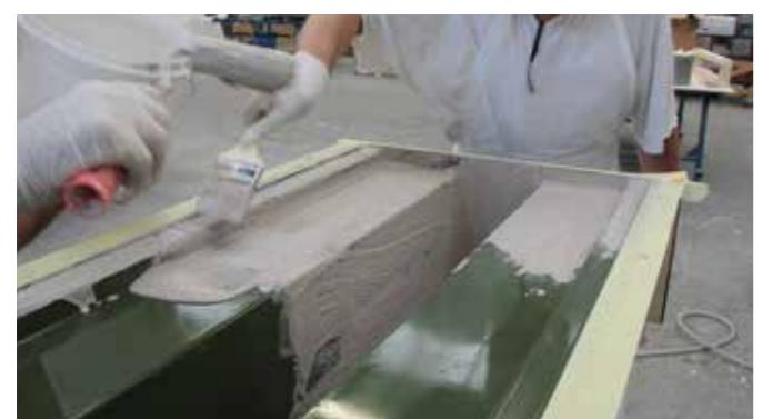
Applying A1 with brush and roller.
