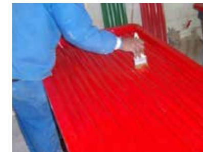
Use a release agent and apply this by brush. After applying wipe out with a cloth.
