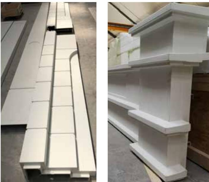
After curing an aluminum mounting structure is connected to the back of the panel by laminating. Including the mounting structure the elements have a surface weight of 20 kg/m<sup>2</sup>.
