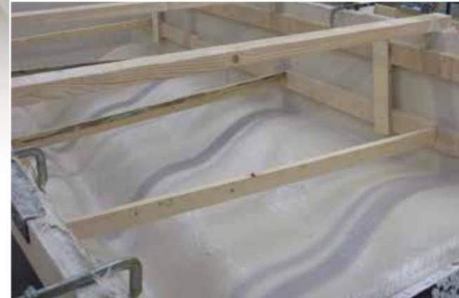
Element laminated and 36 mm plywood beams positioned to the sides
