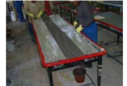
Apply the 1st laminate layer: A1 with 2 layers of A1 Triaxial fibre.
