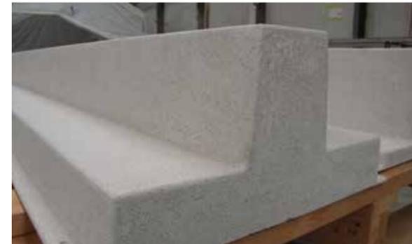
After complete curing, the panels are lightly sand blasted.
