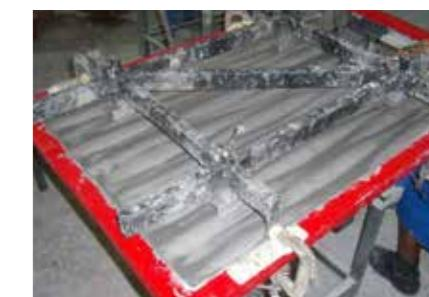
A frame is used to position the mounting brackets on the finished laminate.
