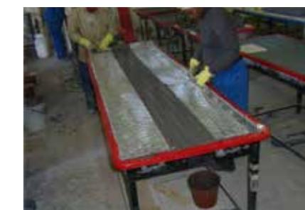
Apply the 1st laminate layer: A1 with 2 layers of A1 Triaxial fibre.
