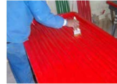
Use a release agent and apply this by brush. After applying wipe out with a cloth.
