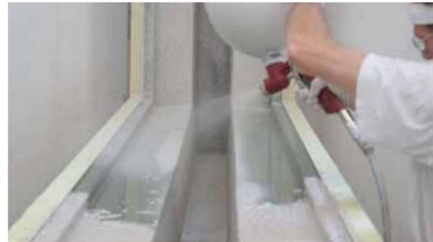
L-shaped panels are sprayed with A1.
