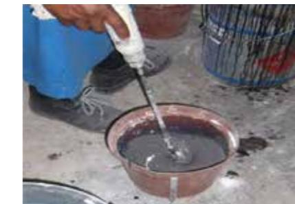
Mix the materials for the gelcoat layer: 50 parts zinc : 100 parts A1 (pbw).
