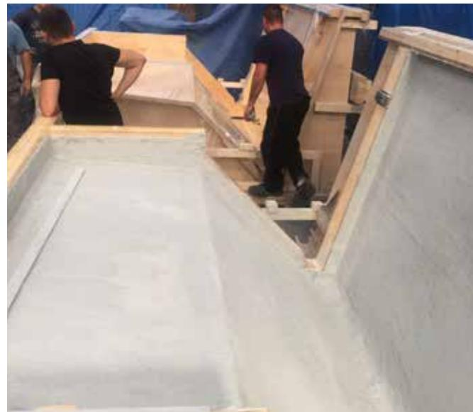
A1 element laminated in the mould
