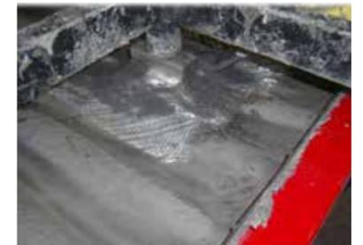
3 layers of A1 Triaxial fibre is laminated on the brackets to get a strong connection.
