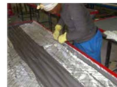
Apply the 2nd layer: A1 with 2 layers of A1 triaxial fibre.
