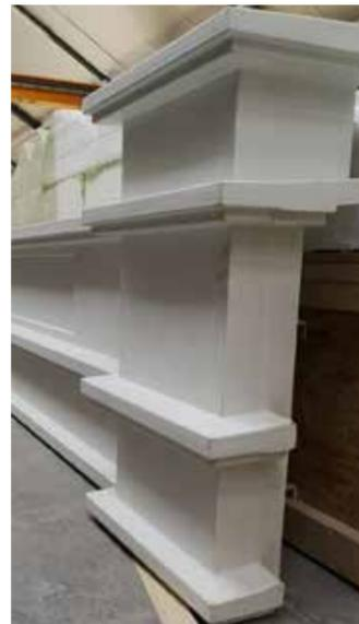
After curing an aluminum mounting structure is connected to the back of the panel by laminating. Including the mounting structure the elements have a surface weight of 20 kg/m<sup>2</sup>.
