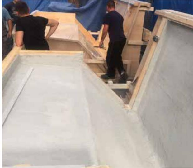
A1 element laminated in the mould
