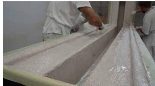
Applying several layers of A1 with Triaxial fibre.
