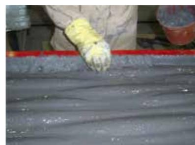
Apply the core layer; A1 met chopped fibers. The core layer has a total thickness of 3 mm.
