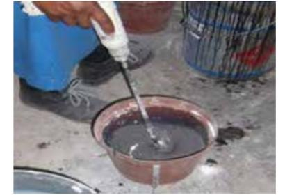
Mix the materials for the gelcoat layer: 50 parts zinc : 100 parts A1 (pbw).
