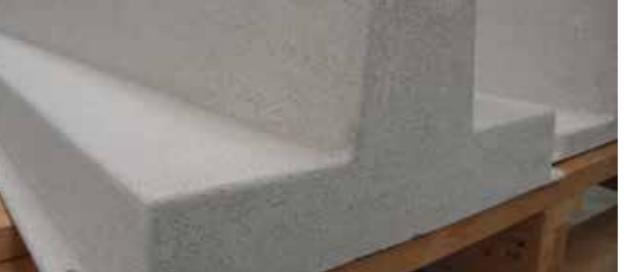
After complete curing, the panels are lightly sand blasted.
