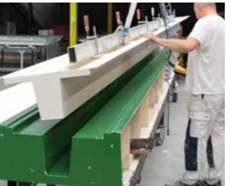
Within 2 hours the panel is demoulded for further curing.
