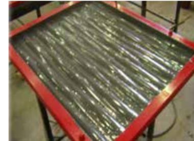
Apply the first layer, this is called the gelcoat layer.
